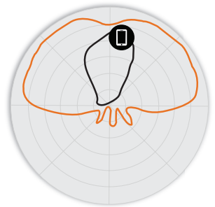
Figure 5 - T310d 5GHz Elevation Antenna Patterns
